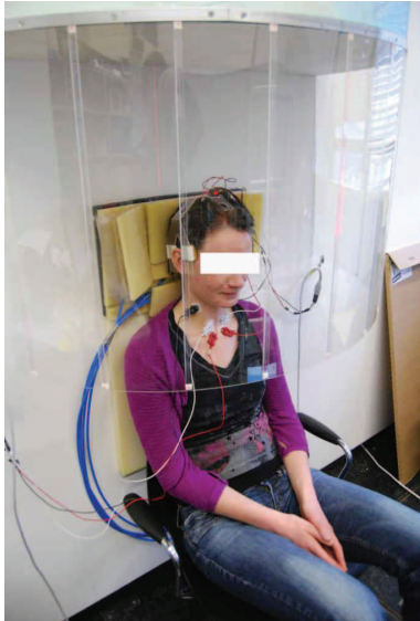
Figure 2. The participant sitting inside the head rotation angle apparatus.
