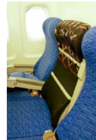
Fig. 2. FSR sensors on head rest area
