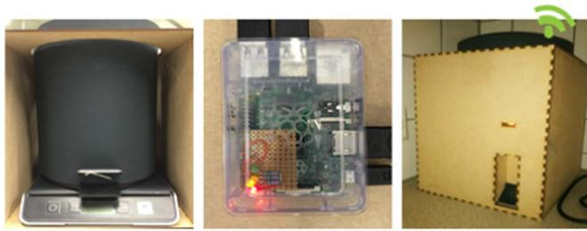
Fig. 6. The augmented bin with USB postal scale and a Raspberry Pi to receive and send data to a server.
