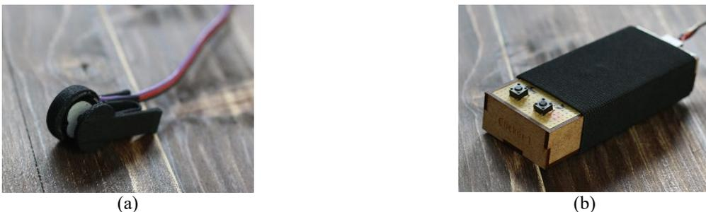
**Figure 2.** (a) Pulse sensor finger clip and (b) the clicker for reaction time measurement.
