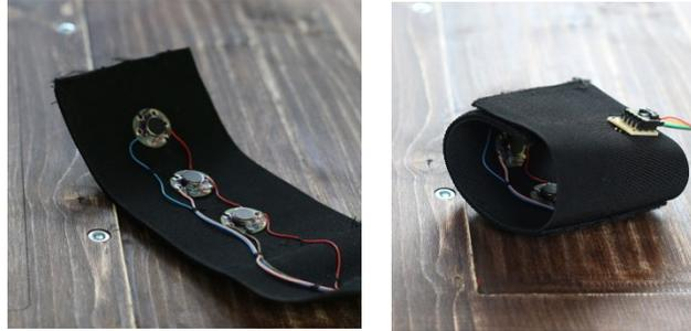
**Figure 3.** The vibration motors attached to the stretchable fabric.
