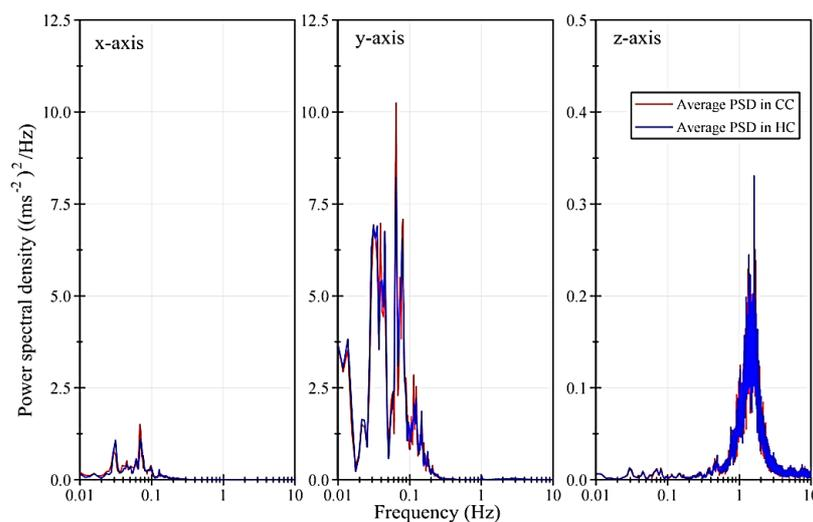
Figure 7. Mean acceleration power spectral densities in fore-and-aft (x-axis), lateral (y-axis) and vertical (z-axis) for both conditions.
