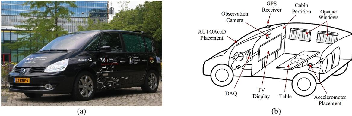
**Figure 1.** (a) The instrumented car Mobility Lab; (b) The layout inside Mobility Lab [35].
