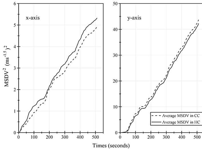
**Figure 8.** Mean accumulated squared motion sickness dose value (MSDV<sup>2</sup>) in the fore-and-aft and lateral directions in CC and HC.
