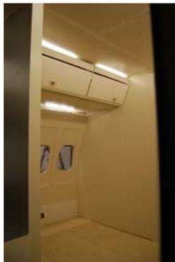
Figure 7 The internal side window panels
