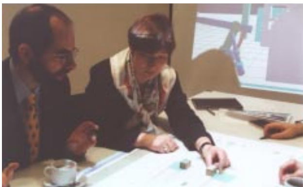
FIGURE 1: BUILD-IT offers a plan view for combined action and perception and a side view with a perspective of the situation.
