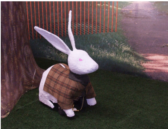
Fig. 2. The ‘White Rabbit’ robot in the park environment surrounded by a 360 degree canvas print of a real park scene nearby Oxford (UK) with backlighting.
