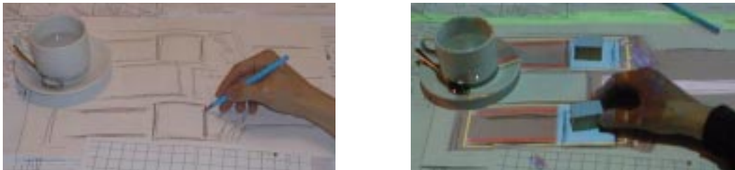
Figure 3. AR means that a real workspace (left) is augmented, or enriched, by a virtual world (right). Even when users interact with the projected, virtual objects, they do not leave the real world context (e.g. sketching) and tools (e.g. pencil).
