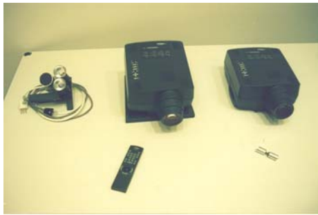
Figure 2: Detailed view of camera, lamp, beamers with remote control and adjustment screw (left). All these parts have appropriate places for installation in the rack (right). Computer and keyboard are put into the lower part of the rack.
