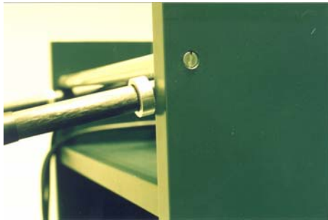
Figure 9: Move the mirror suspension backwards or forewords (left) so that that the light field is centred on the mirror (right).
