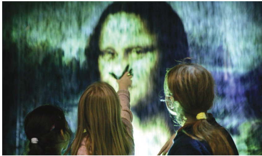
FogScreen technology, invented by two Finnish researchers, projects an image onto a display surface of water vapor diffused into the air as a very dry fog. Viewers can even put their hands through the images.
