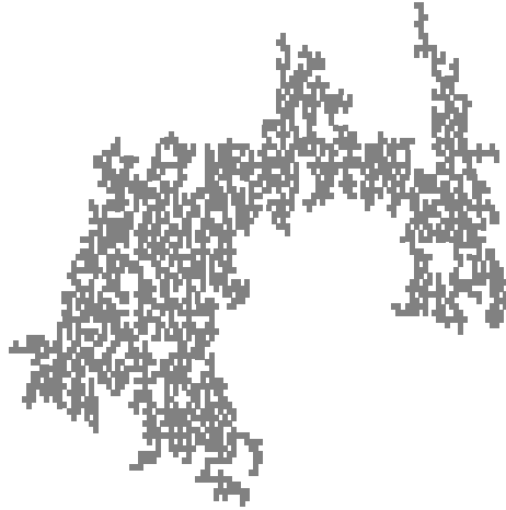
Fig. 6.41. Example of a cluster of invaders obtained on a square lattice after 2,000 iterations of the invasion rule
