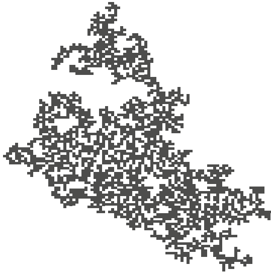
Fig. 6.16. Grassberger's general epidemic process. The cluster represents the spread of the epidemic to 4,000 sites for p = 0.6
