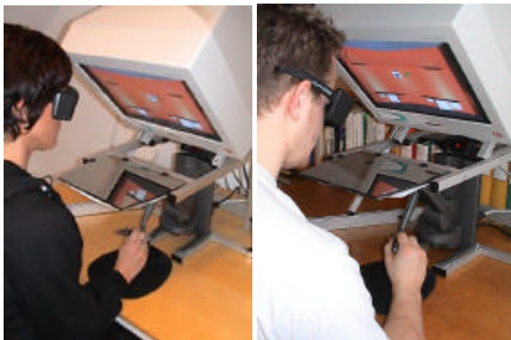
Figure 1: Two persons collaborating in the virtual environment using the ReachIn Display system.
