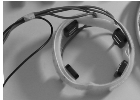
Figure 2: The device prototype for attaching EMG electrodes.
