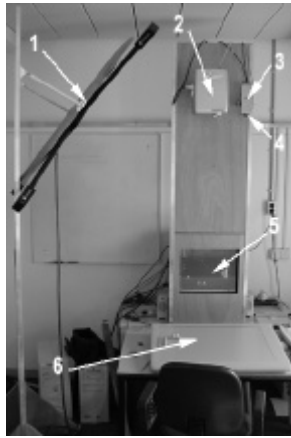
Figure 1: Visual Interaction Platform. 1-3D tracker, 2-LCD Projector, 3-Camera, 4-Infrared light source, 5-CRT screen (Communication Space) 6- Wacom Tablet with projection image (work space).
