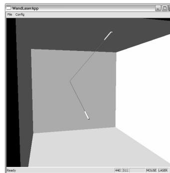
Figure 4: Software system illustrating XWand (lower white cylinder) and WorldCursor device (upper white cylinder), where room geometry is known.
