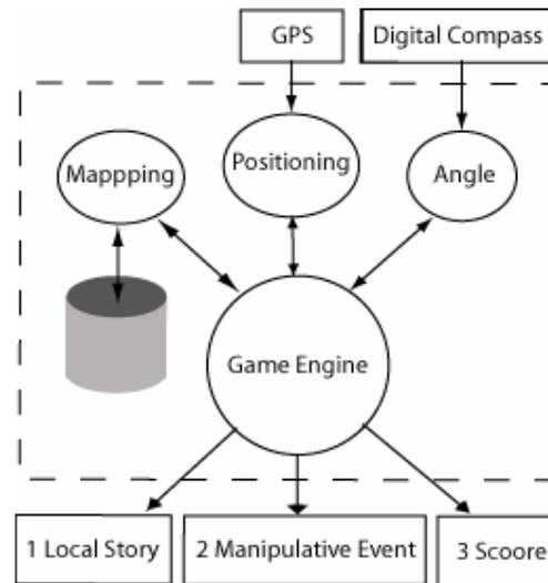
Figure 9: System architecture
