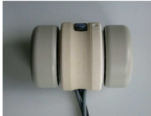
Figure 3: The YoYo with a cylindric centerpiece and a single button.
