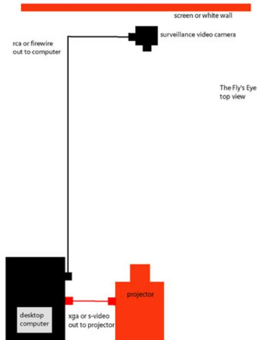
Figure 2: Basic technical configuration of the installation
